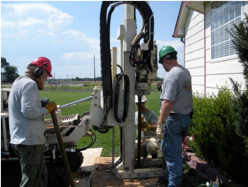
**Figure 2.** Photograph of track-mounted Geoprobe™ rig adjacent to a house in Valley Center, Kansas.
