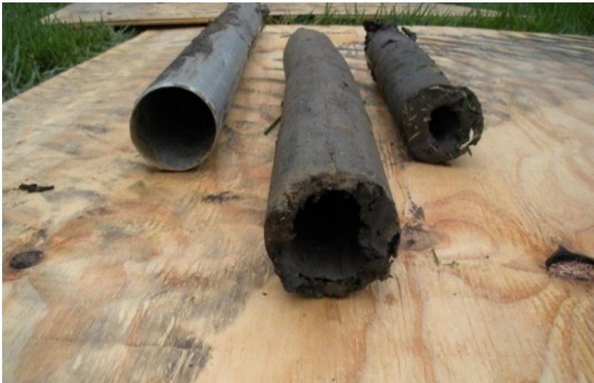
**Figure 6.** Photograph of black clay. Hole in center of clay is from previous push with steel rods containing PVC liners.
