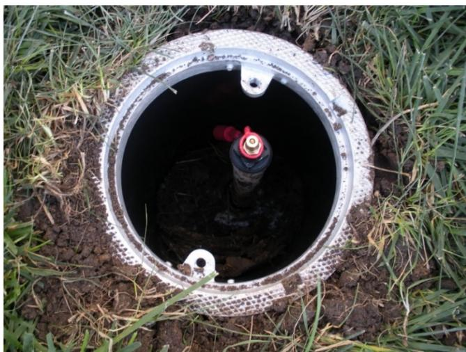
**Figure 10.** Photograph of rubber fitting with brass quick-connect fitting to seal PVC wells.
