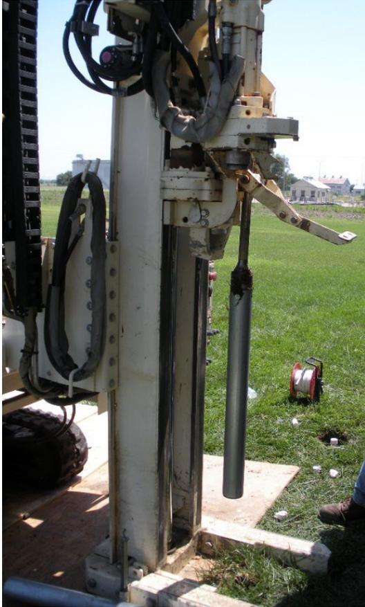
**Figure 5.** Photograph of thin-walled 7.6 cm tube used to enlarge boreholes.
