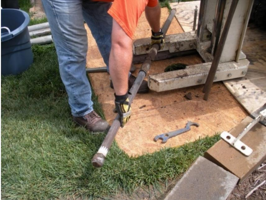
**Figure 3.** Photograph of removal of a PVC liner containing soil and a PVC core catcher.
