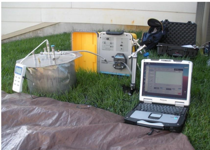
**Figure 12.** Photograph illustrating vacuum testing of fittings associated with leak detection chamber
